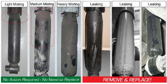
Misting is normal for hydraulic shocks. Misting presents as a thin all over covering or film on the shock under the dust tube. LEAKING will present as streaks and uneven runs of oil under the dust tube and the shock should be replaced.
